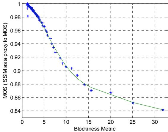
Figure 6 Scatter plot of ssim against the blockiness metric b1 for matlabtm jpeg codec on sine-squared grey scale-radial test pattern
