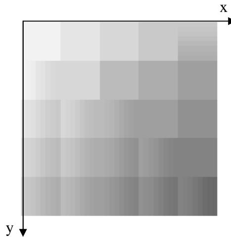
Figure. 5 Blockiness resulting from JPEG codec at high compression ratio.
