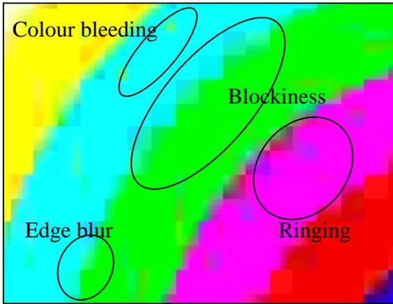
Figure. 3 Coding artefacts around the colour edges resulting from a JPEG codec on 1:120 compression
