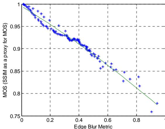
Figure 7. scatter plot of ssim against the blur metric for Matlab™ JPEG codec on monochrome-rings test pattern
