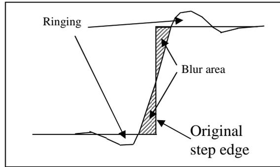
Figure. 4 Ringing and edge blur at an edge of a one-dimensional signal.
