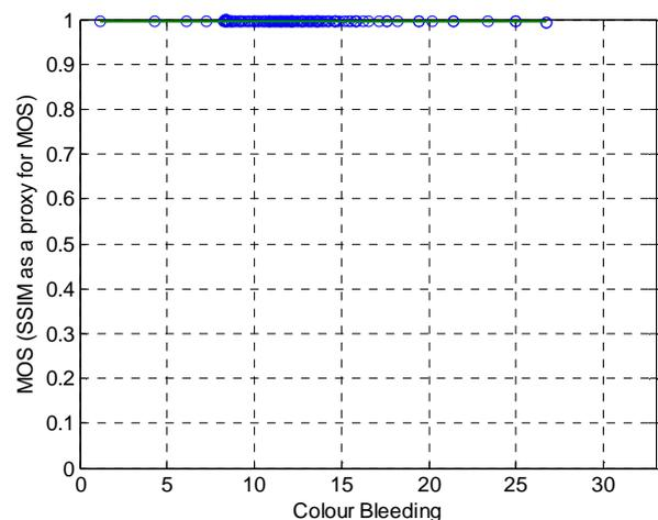
Figure 8. scatter plot of mos against the colour bleeding metric (hue spread) with the data set based on honeycomb test pattern
