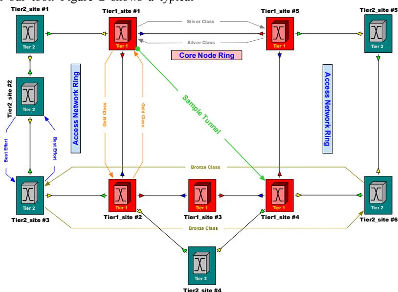
Figure 2: Sample network showing nodes, links, traffic streams and tunnel objects
