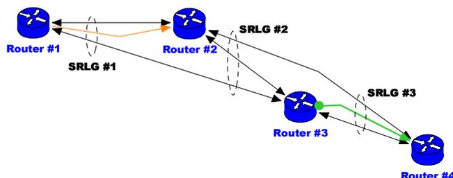
**Figure 3: Network model showing SRLGs**
