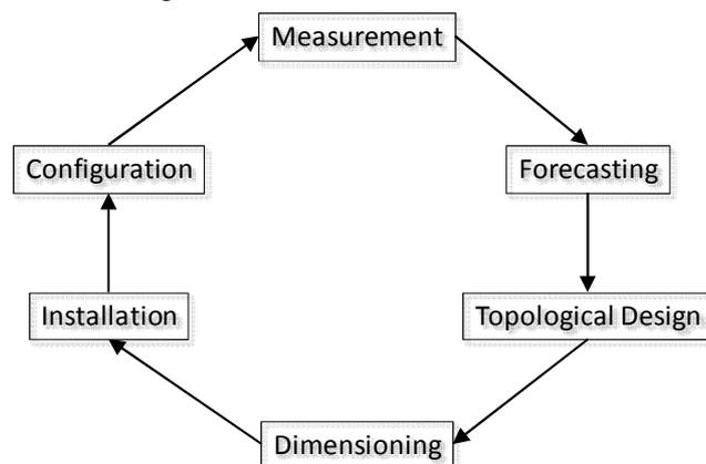
**Figure 1: Planning and Installation Cycle**
