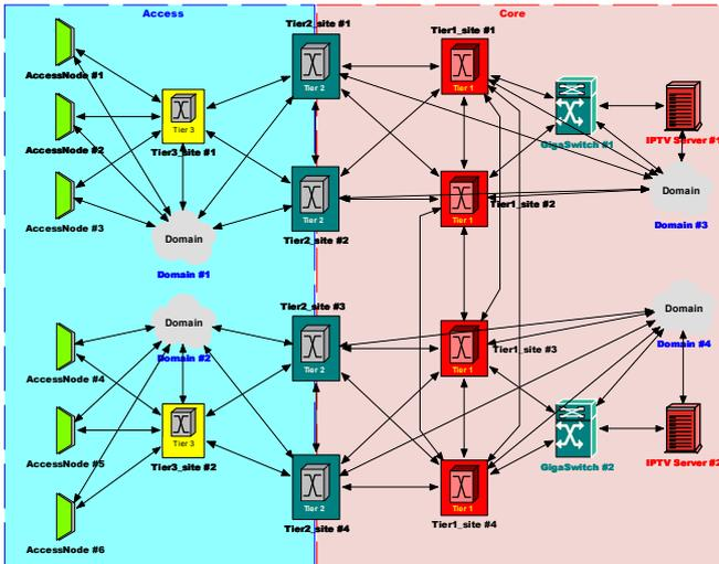
Figure 5: Sample network showing a simplified study of the connections to an IPTV server
