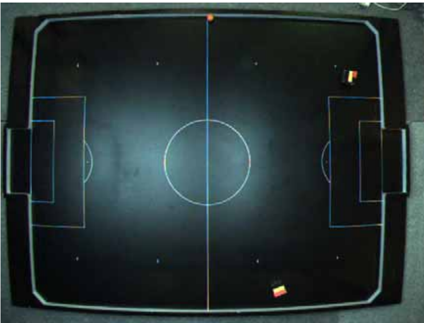
Fig. 1. Example field, clearly showing lens distortion and mild perspective distortion.
