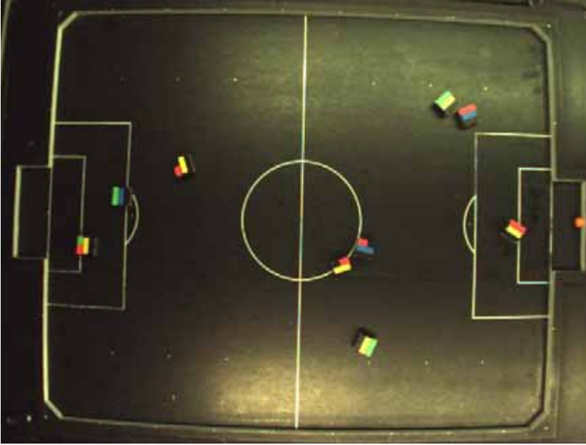
Fig. 5. As a result of lighting and specular reflection, the edge of the playing area may be harder to detect.
