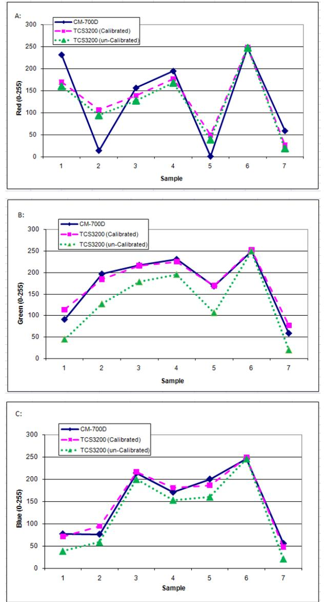
Figure 6. TCS3200 sensor *RGB* readings, calibrated and un-calibrated, compared with the CM-700D readings of: Red (A); Green (B); Blue (C). (Colour samples are as given in Table II)
