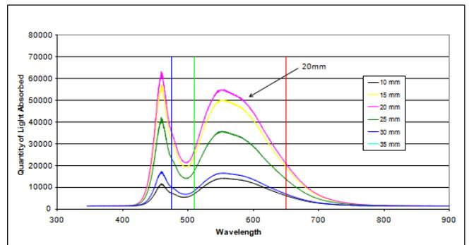
Figure 4. Light absorbed from TCS3200 across the white LED light spectrum when the sensor is positioned at 6 different heights.
