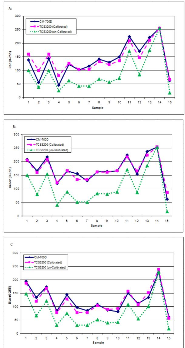
Figure 7. TCS3200 sensor RGB readings, calibrated and un calibrated, compared with the CM-700D readings of: Red (A); Green (B); Blue (C) for a range of RHS green colours. (Colour samples are as given in Table V)
