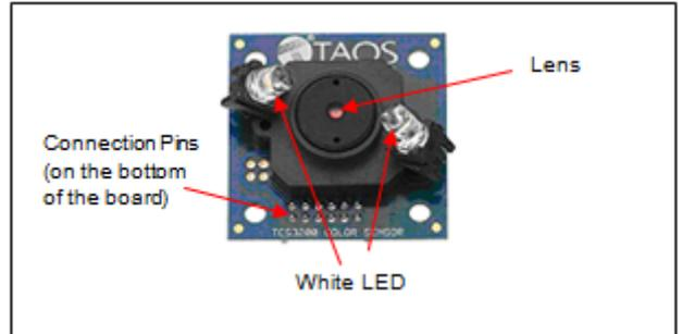
Figure 3. Parallax TCS3200 colour sensor.
