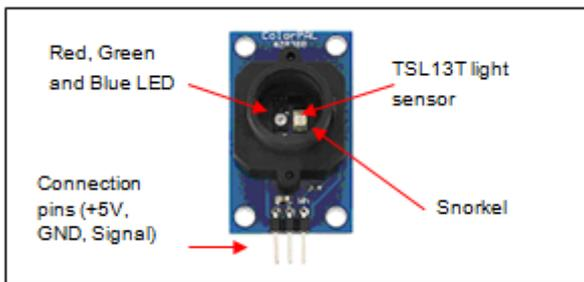
Figure 2. Parallax ColorPAL colour sensor.
